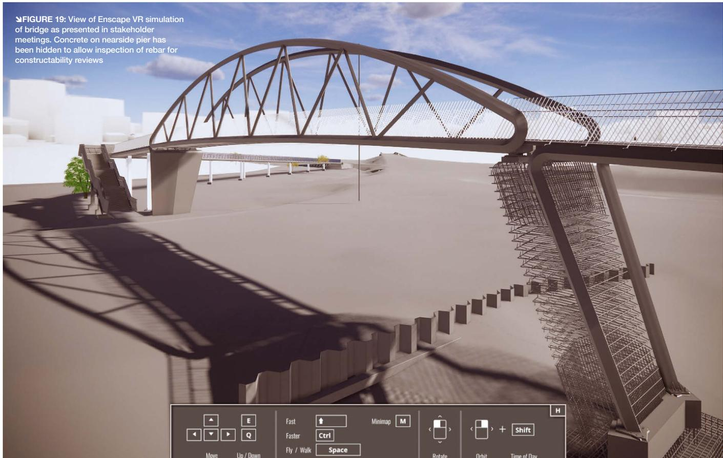
**FIGURE 19:** View of Enscape VR simulation of bridge as presented in stakeholder meetings. Concrete on nearside pier has been hidden to allow inspection of rebar for constructability reviews
