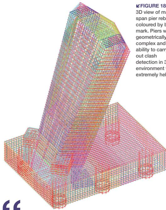
**FIGURE 18:** 3D view of main-span pier rebar, coloured by bar mark. Piers were geometrically complex and ability to carry out clash detection in 3D environment was extremely helpful
