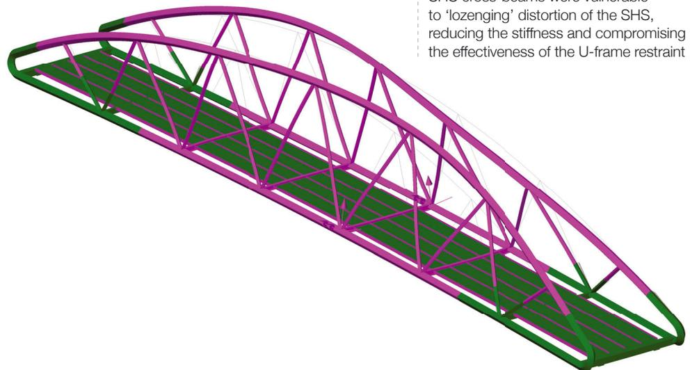
of geometrically non-linear (large displacement) elastic analyses to BS EN 1993-2 Annex D. The initial imperfections were scaled by the values outlined in Table D.9 for the worst-case buckling curve d (i.e. 140mm for a half sinusoidal wave buckling mode and 190mm for a full sinusoidal wave buckling mode).
