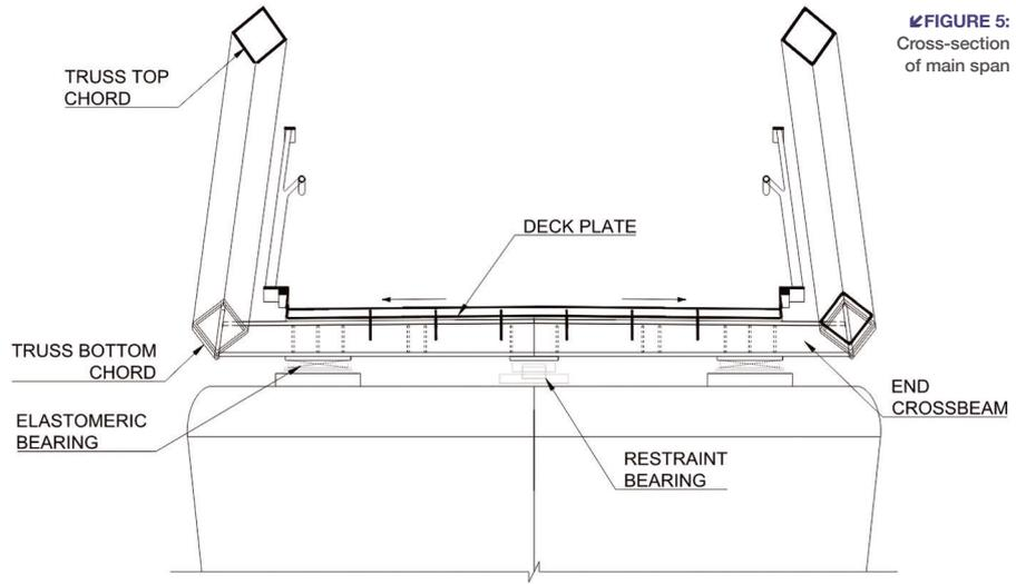
FIGURE 5: Cross-section of main span
