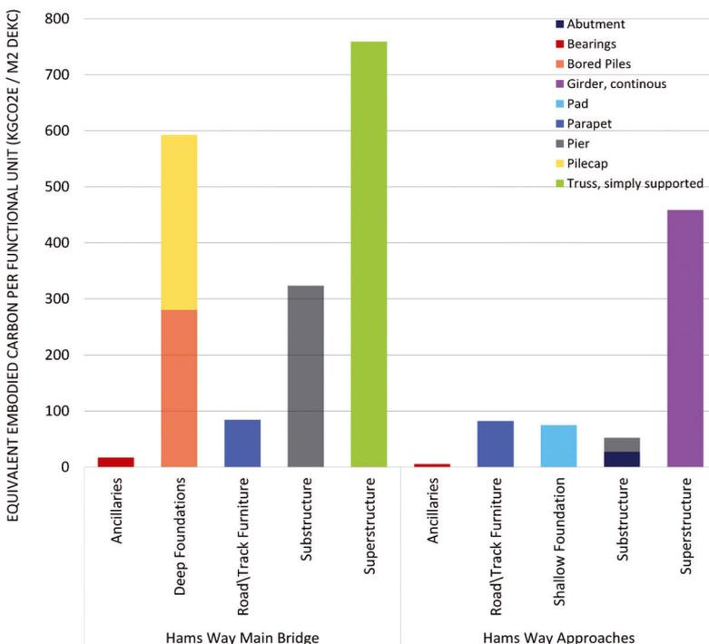
↑ **FIGURE 20:** Summary of equivalent embodied carbon (lifecycles A1–A5) per square metre of usable deck area
